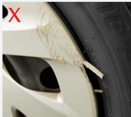
Cracked wheel trim
